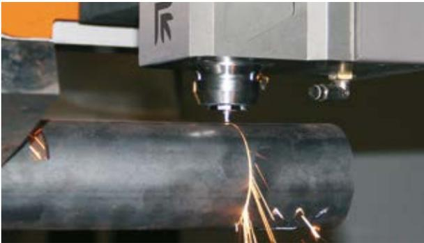
Platino easily switches to tube cutting.
