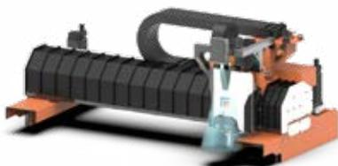
Automatic edge or profiles detection function to support users during the cutting preparations using a camera system to recognize the precise position of the loaded blank. The measuring software allows taking highly accurate (< +/- 0.15 mm) references on the sheet metal thanks to a high definition camera.
