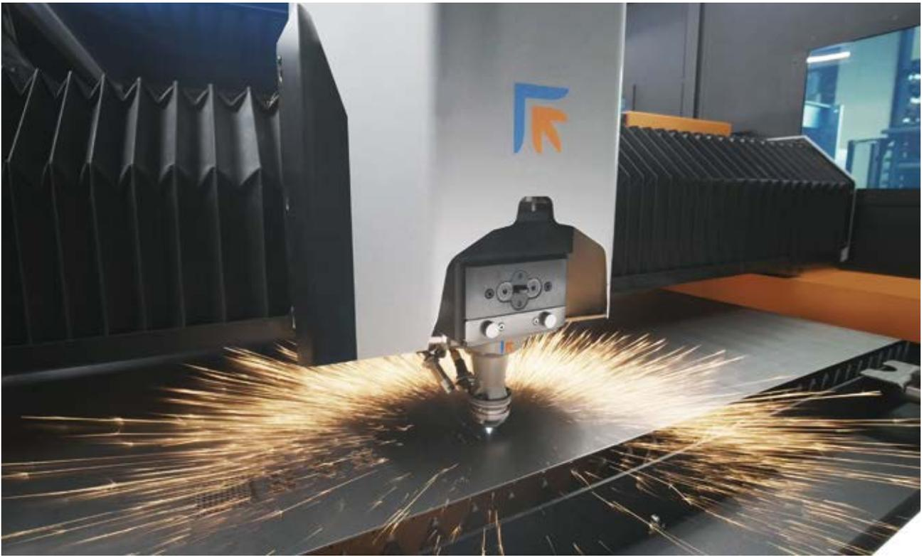
Best-in-class dynamics to grant low cycle times with excellent cutting quality. Laser Genius+ can process with high quality levels a wide range of materials up to 30mm and can be equipped with laser generator with powers ranging from 2 to 15 kW.
