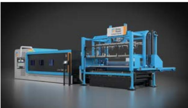
The Laser Genius+ can be integrated with a wide range of automation solutions that perform functions such as material loading/unloading, storage and part sorting automatically.
