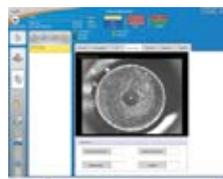
New dedicated device monitoring, through camera positioned on the axis of the tip exit hole, both centering and nozzle status. The device, thanks to the checks of the nozzle status and beam centering, helps to ensure reliability and saves waste of time.
