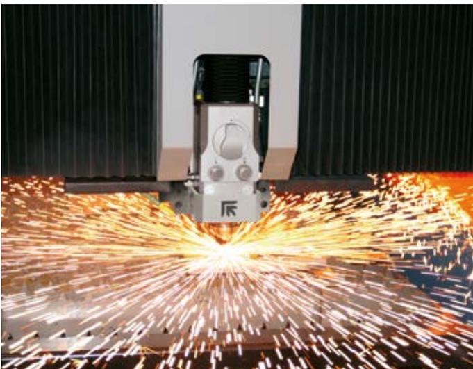
Prima Power CO<sub>2</sub> head features safe impact protection system, process gas pipe, wide range of nozzles, F axis for controlling the focal position independently of the Z axis, lens drawer (for 5" or 7,5" lenses), capacitive sensor for automatically maintaining the preset stand-off from the sheet metal.
