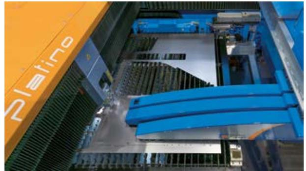
Platino equipped with LST for part sorting and stacking.
