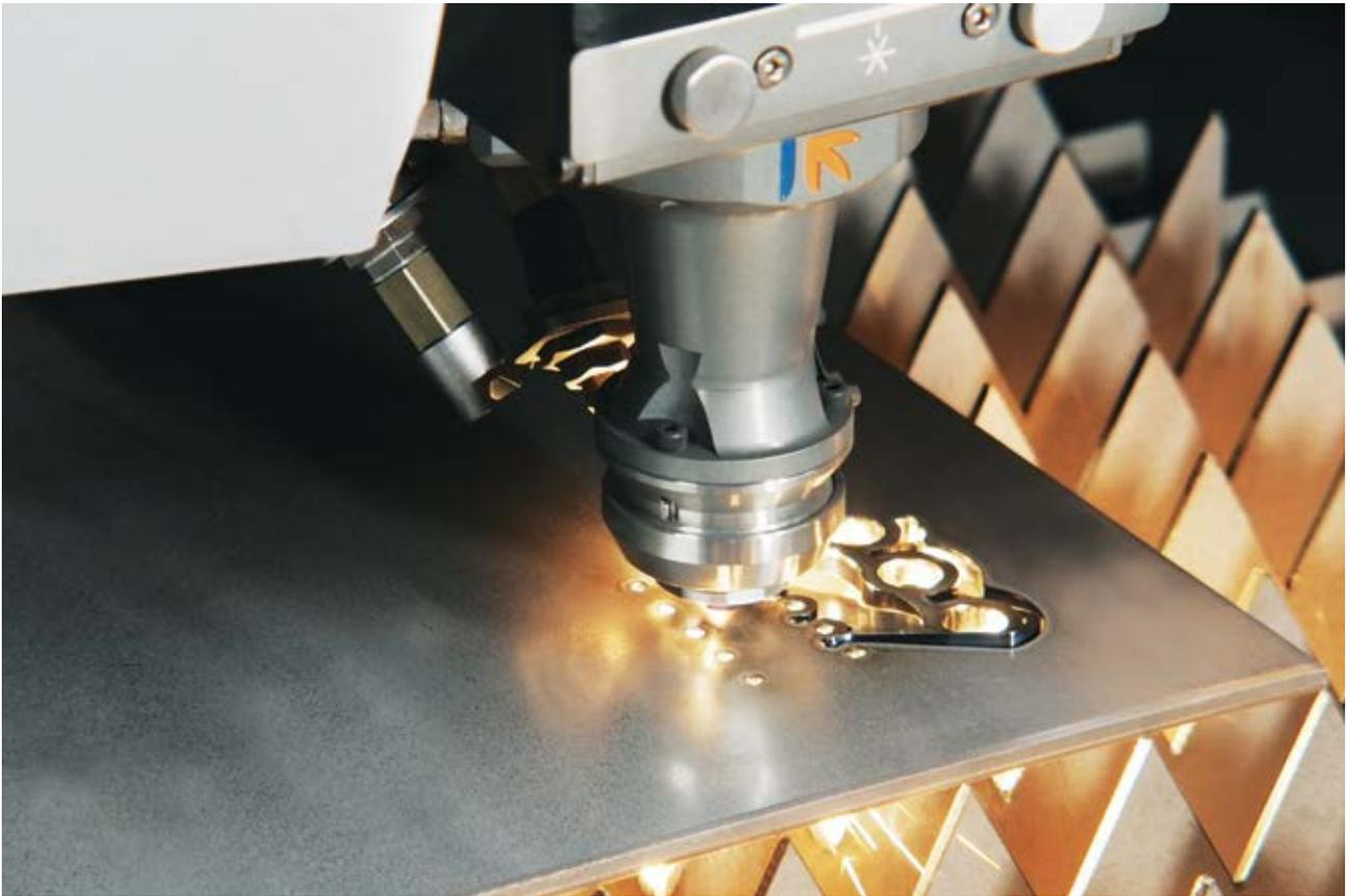
Laser cutting is an amazingly flexible technology. A wide variety of materials and thicknesses can be processed, with no limit to the shape you can obtain. Its programming is so fast that any change can be applied in any phase of your production with virtually no extra costs and time. Its precision is the highest, the quality of the cut edge is excellent and there is no part distortion.
